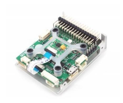
With ingenious design MindPX packs a built-in vibration damping structure into such a compact space.
